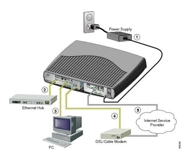
How To Setup A Cisco Router
